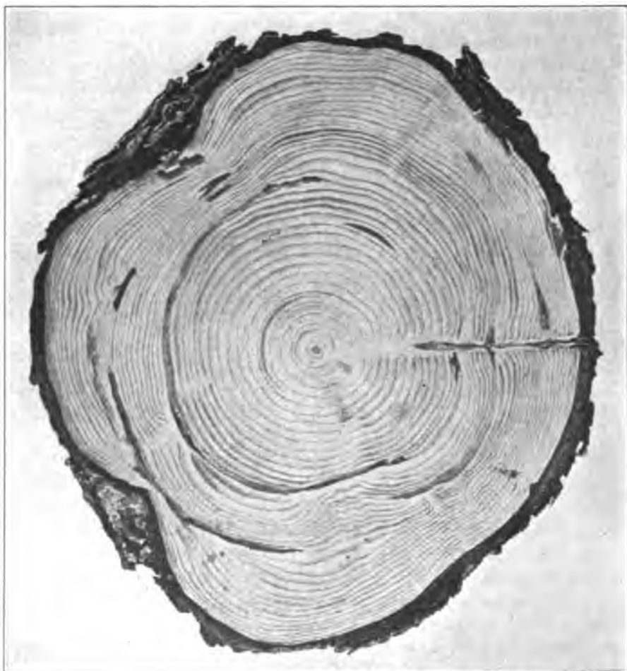
Fig. 98. Cross-section through a spruce with numerous overgrown wounds due to lightning. (After Hartig.)
